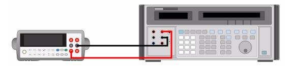
For range  $\geq 1$  A , Input  $\geq 3$ A
