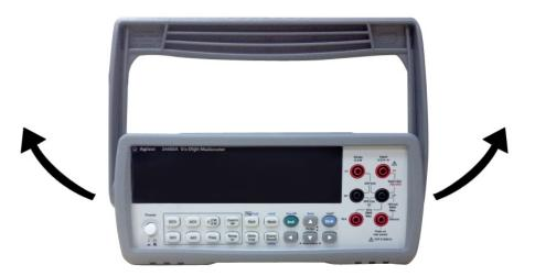
**3** Remove the instrument bumpers. Pull from a corner and stretch the bumpers off the instrument.
