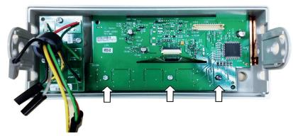
**2** Pull the rubber keypad from the plastic housing.
