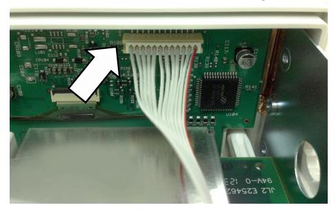
7 Disconnect the ribbon cable connectors from the front panel.
