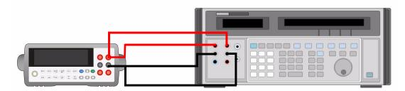
2-W resistance without compensation (For range 1 M $\Omega$   $\sim$  100 M $\Omega$  )
