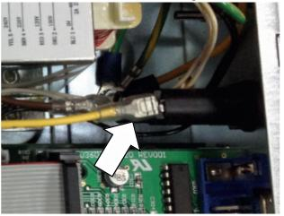
**9** Disconnect the fuse wire as shown in the figure below:
