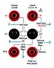
**Note:** The front-panel terminals and current protection fuse are shown above.
