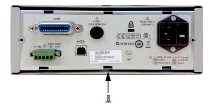
**5 Remove the cover.** Remove the screw in the bottom of the cover and slide the cover off the instrument.
